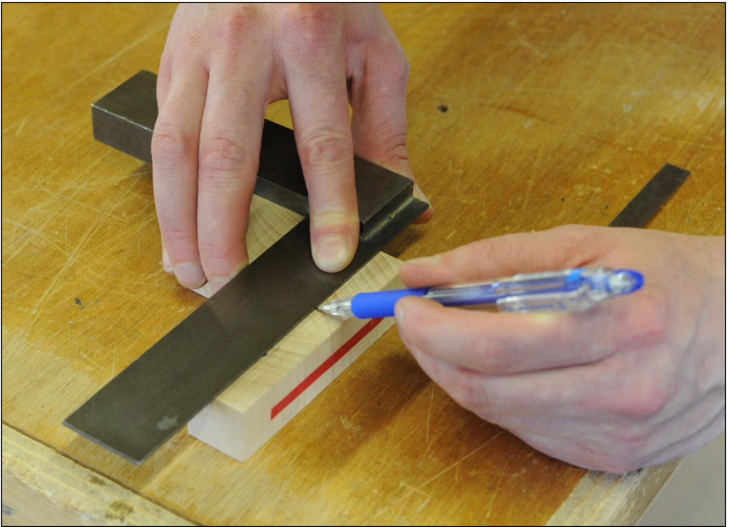
Using a square from the belly rail edge, mark the cut line through the bushing cloth mark.
