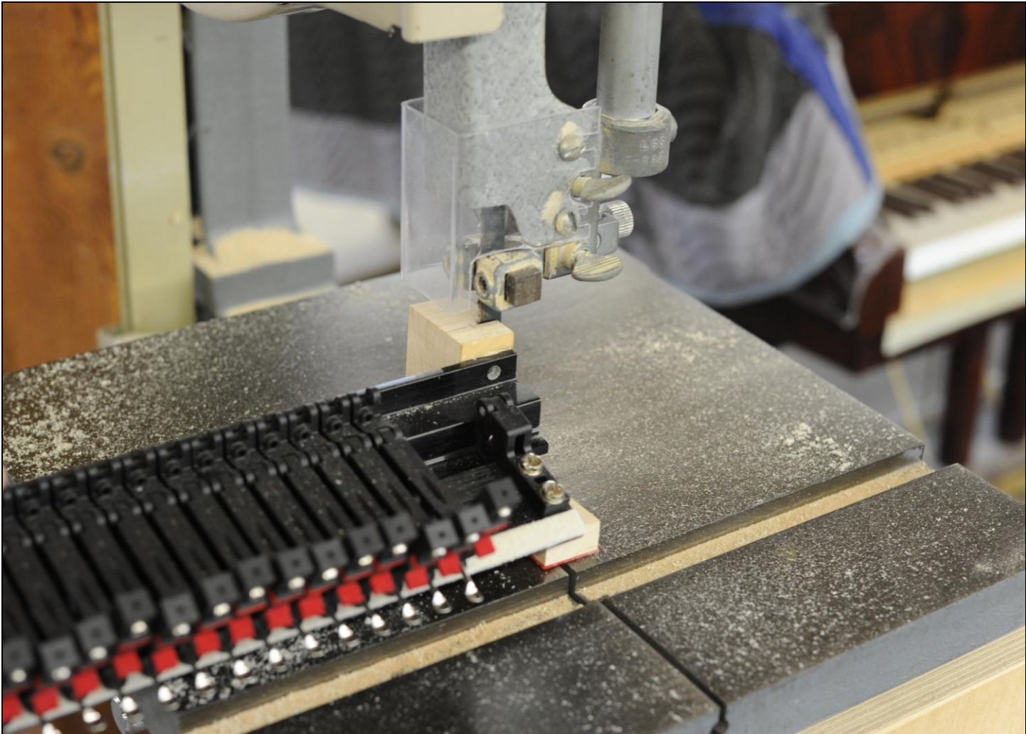
On a band saw cut the back side of the line.
